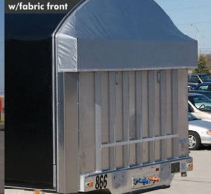
DOT Bulkhead w/fabric front
